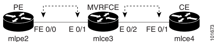
Figure 6-1 MVRFCE PE-CE Link
