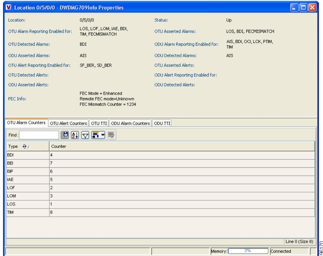
**Figure 14-3** shows the tabs that are displayed in the G709 Info Properties window for Cisco 7600 series devices. For Cisco 7600 series devices:
