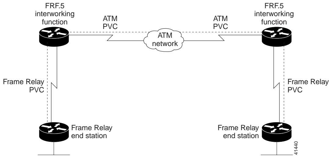
FRF.5 describes network interworking requirements between Frame Relay Bearer Services and Broadband ISDN (BISDN) permanent virtual circuit (PVC) services.
