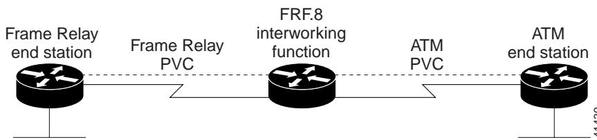
FRF.8 describes a one-to-one mapping between a Frame Relay and an ATM PVC.
