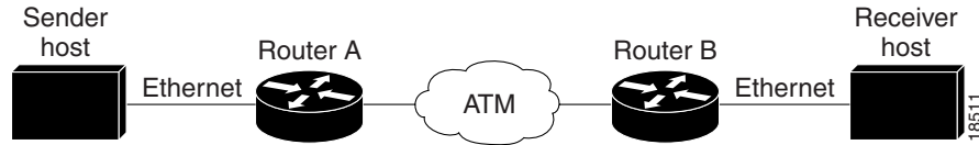
Figure 24 Example RSVP-ATM QoS Interworking Configuration
