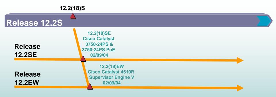
Derived from Release 12.2(18)S, Releases 12.2SE and 12.2EW provide Release 12.2S functionality and new features and hardware for the Cisco Catalyst 2970, 3750, and 4500 Series Switches
