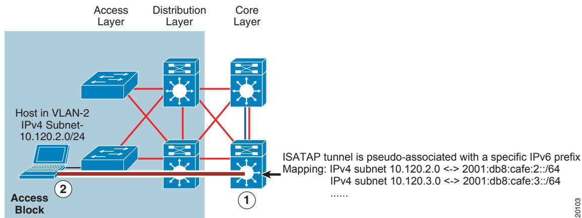
1. The core layer switch is configured with a loopback interface with the address of 10.122.10.2, which is used as the tunnel source for ISATAP, and is used only by users located on the 10.120.2.0/24 subnet.
