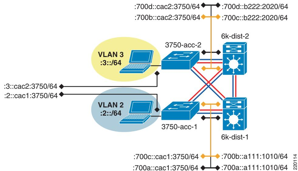
Figure 13 shows that the links between the access layer and distribution layer are now routed links instead of trunked Layer 2 links. IPv6 addressing and routing is configured on the new links, and the hosts in the VLANs use the IPv6 address of the VLAN interface on the access switch as the default gateway. The following configuration example shows the relevant configurations for the 3750-acc-1 and 6k-dist-1 switches.
