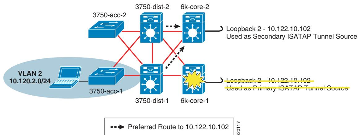
The updated routing table entry for 10.122.10.102 on the distribution layer switches is as follows:
