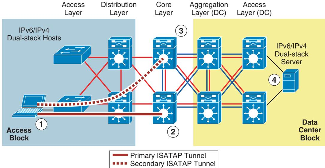
1. The host establishes an ISATAP tunnel to the core layer.
