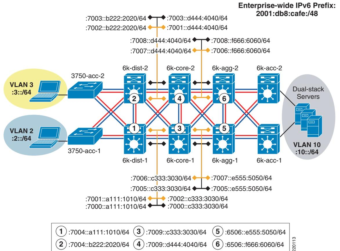
In addition to the physical interfaces, IPv6 addresses are assigned to loopback and VLAN interfaces. Table 6 shows the switch, interface, and IPv6 address for the interface.
