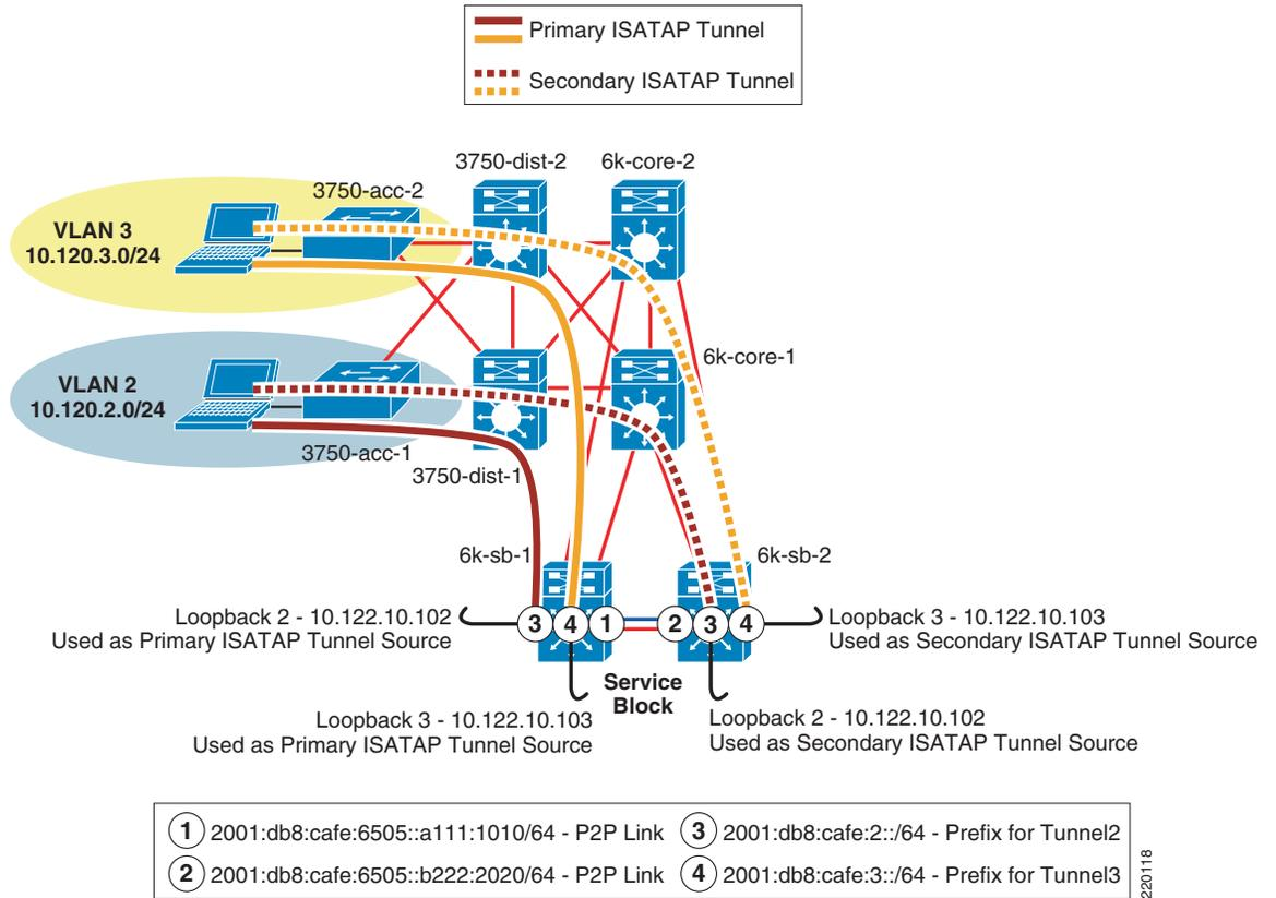
Figure 18 shows the manually-configured tunnel topology for the SBM. The topology diagram shows the loopback addresses on the service block switches (used as the tunnel source for configured tunnels) and the IPv6 addressing used on the manually-configured tunnel interfaces.
