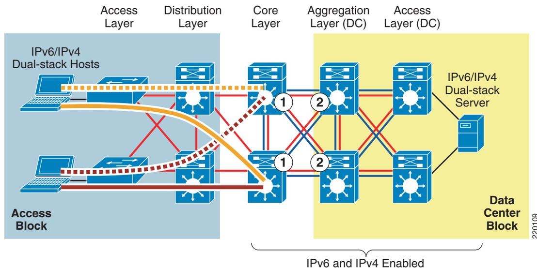
1. In HME1, the first place to implement classification and marking is on the egress interfaces on the core layer switches. As was previously mentioned, the IPv6 packets have been tunneled from the hosts in the access layer to the core layer, and the IPv6 packets have not been “visible” in a decapsulated state until the core layer. Because QoS policies for classification and marking cannot be applied to the ISATAP tunnels on ingress, the first place to apply the policy is on egress.
