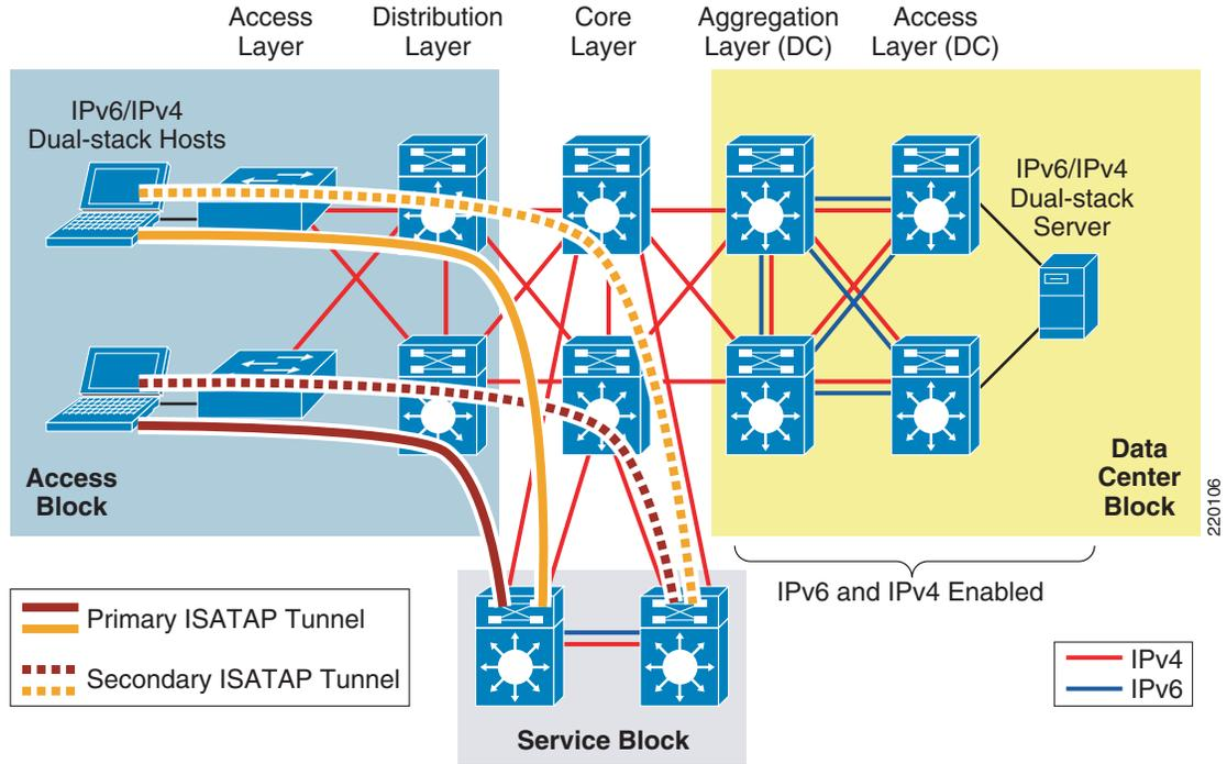
Figure 7 shows the redundant, manually-configured tunnels connecting the data center aggregation layer and the service blocks. Hosts located in the access layer can now reach IPv6 services in the data center access layer using IPv6. Refer to [Conclusion, page 63](#) for the details of the configuration.
