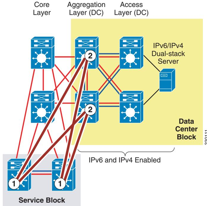
1. The SBM switches receive IPv6 packets coming from the ISATAP interfaces, which are now decapsulated, and can apply classification and marking policies on the egress manually-configured tunnel interfaces.
